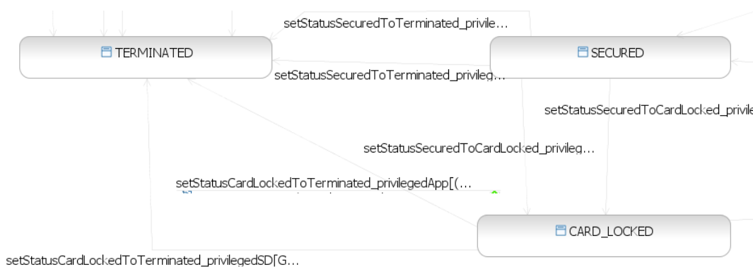
Figure 5.8: A new transition is introduced between Card_Locked and Terminated in V2.2 of the GP
